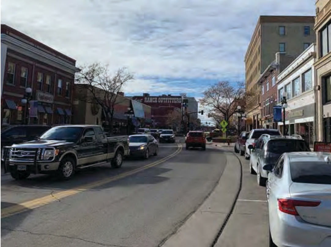
E. 2nd Street in downtown Casper is an example of a chicane
